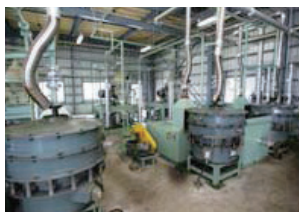
Waste oil treatment (vibration sieving machine)
