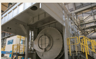
Rotary gas melting furnace (Daiseki MCR) uses LNG instead of coke for recycling lead
