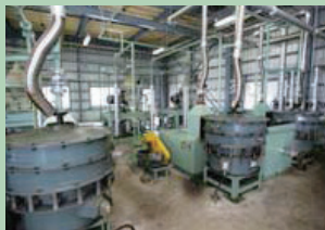
Waste oil treatment (vibration sieving machine)
